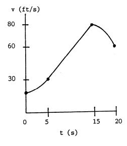
Note that the shape of the v-t curve can be inferred directly from the shape of the a-t diagram. At t=0, the slope of the v-t diagram is zero since a=0. The slope increases in a linear fashion until t=5 s. Between t=5 s and t=15 s, the slope remains constant. At t=15 s, it abruptly changes to zero, and then it decreases linearly.
