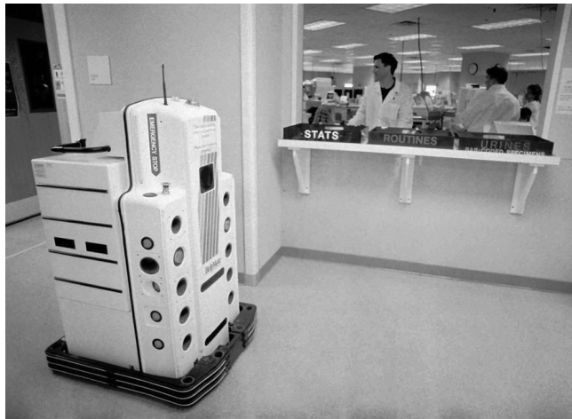
Figure 2.45: Robot for delivery of hospital supplies Source: AP Images
